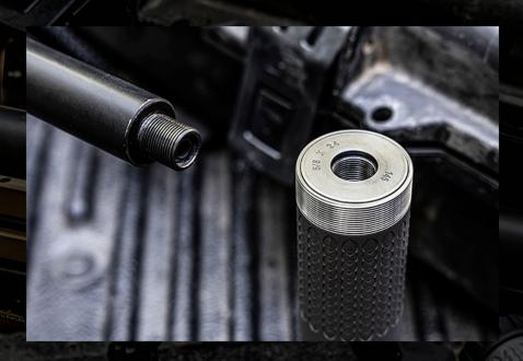
Unscrew the thread mount from the monocore and reinstall desired thread mount, making sure no debris is in the tube or on the threads and mating surfaces of the parts. Insert completed monocore into the tube making sure to line up the notch in the monocore with the keeper pin in the tube, so that the monocore is completey flush as seen above.
