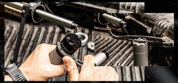
Use the supplied spanner wrench to install or remove either the castle nut or the muzzle brake locking ring.
