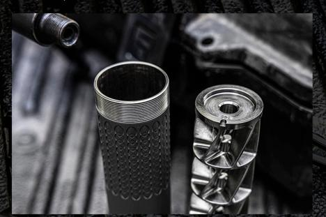
Using the spanner wrench and the tube clamp remove the encapsulator from the forend of the 2nd stage. Remove the tube clamp and use a twisting and pulling motion to remove the tube from the monocore. The monocore can now be unthreaded from the first stage of the suppressor.
